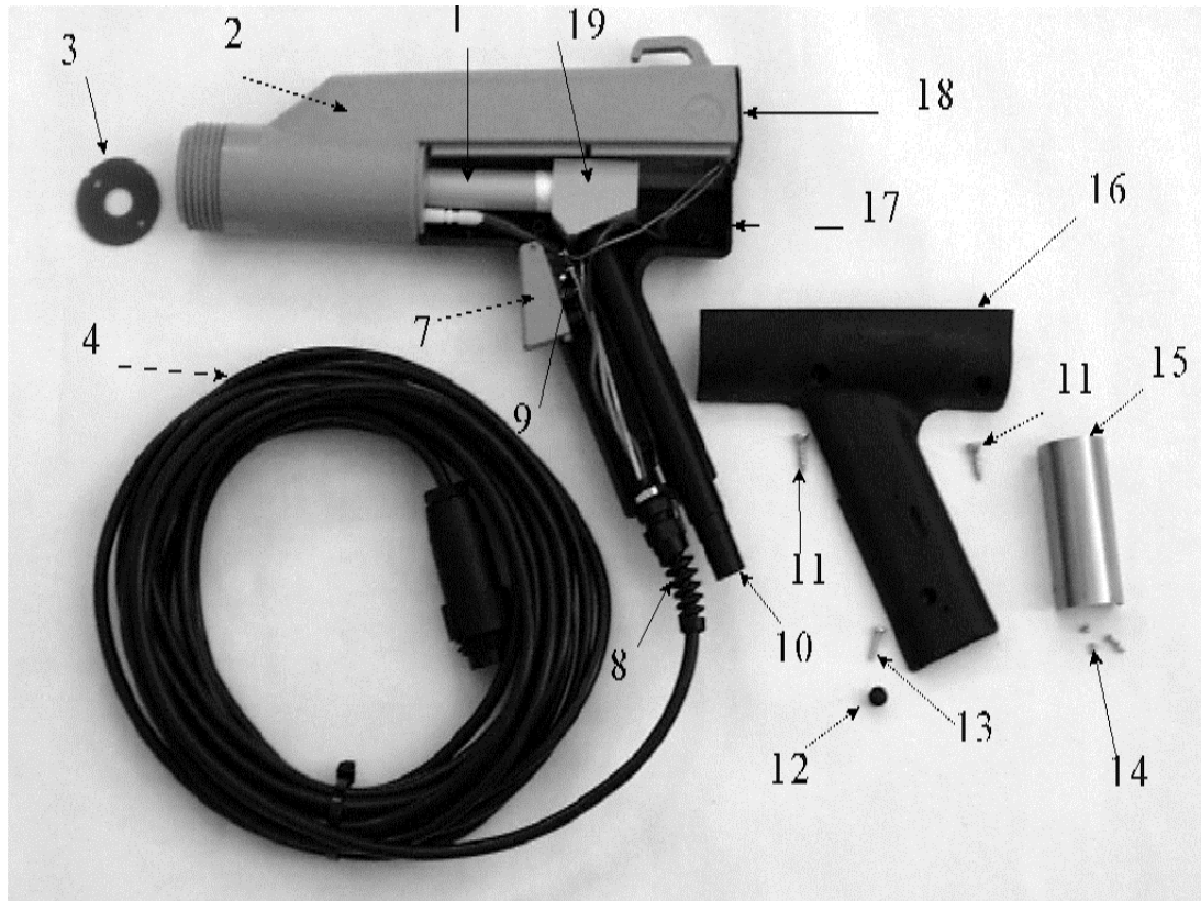
Illustration 6 Overview of a disassembled MG801
