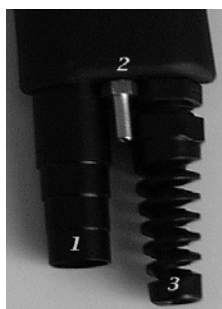
Illustration 9 Connections at the bottom of the gun
