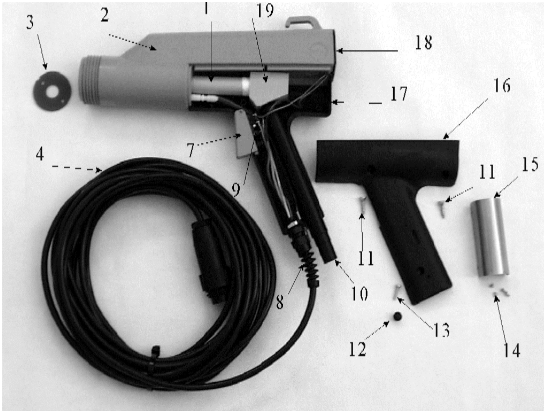
Illustration 7 Overview of a disassembled MG850
